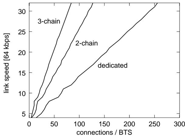
Figure 5: Required Link Speed
