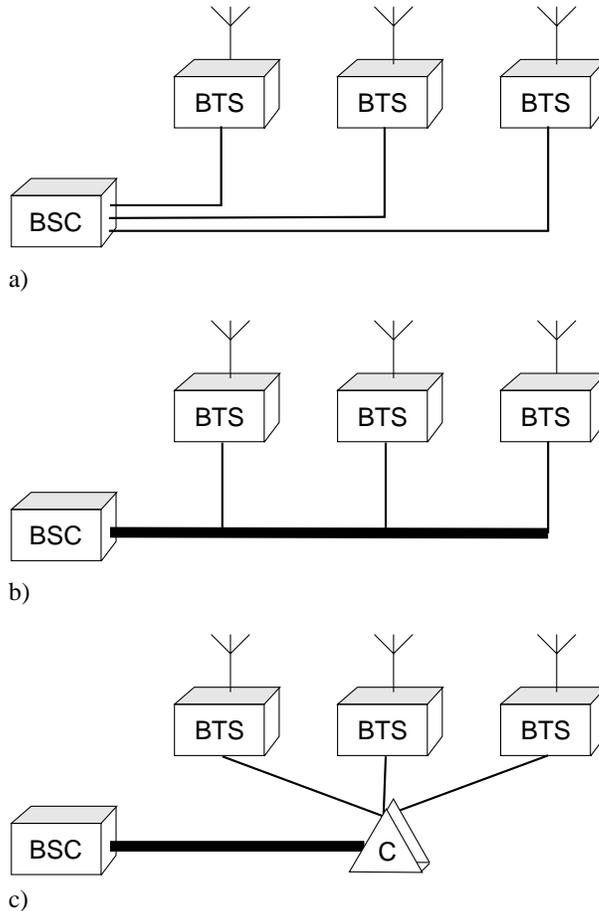
Figure 2: (a) Star, (b) Drop-and-Insert, and (c) Concentrator Architecture
