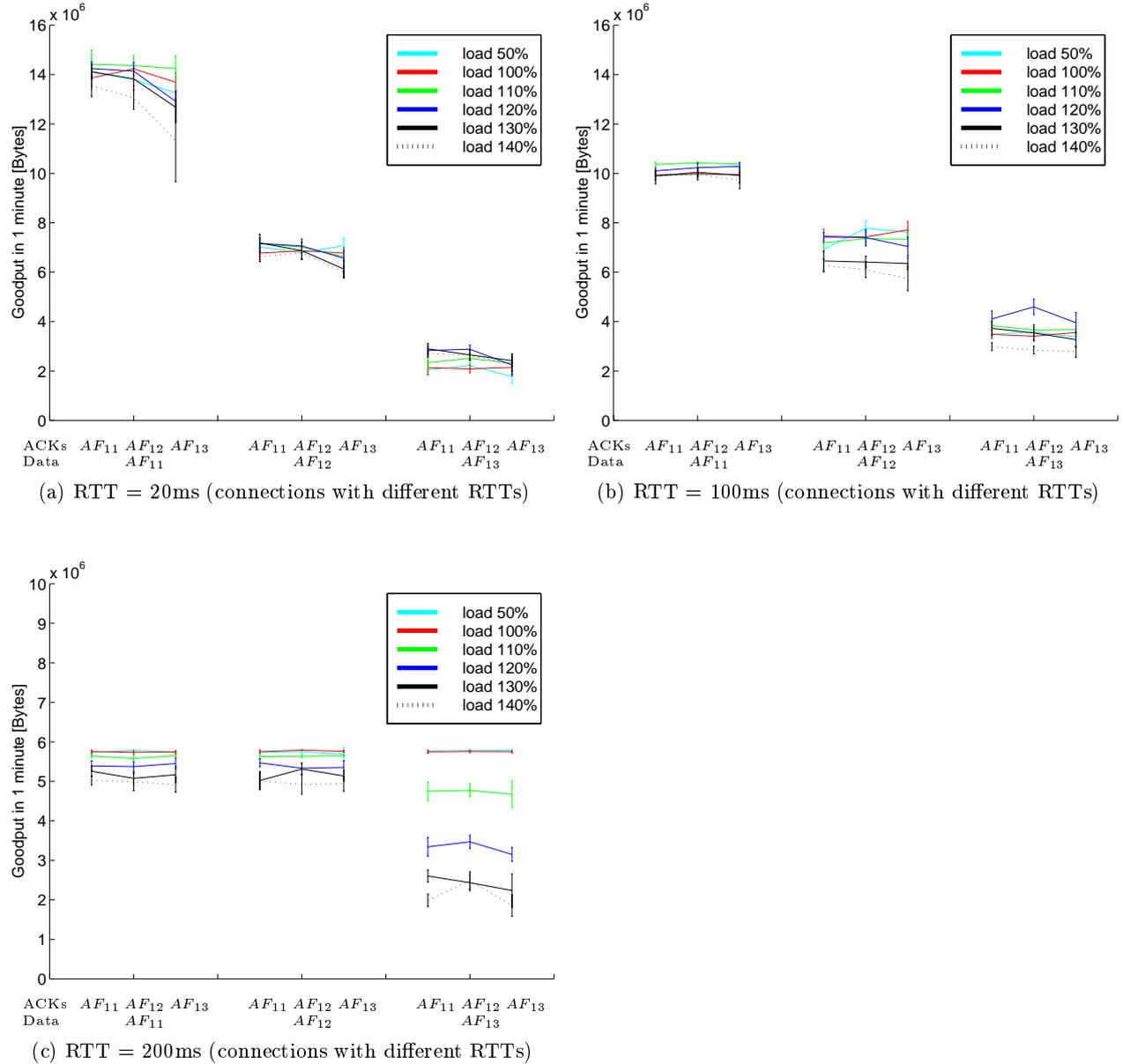
Figure 9: Comparison of goodput for different combinations of drop precedences with varying load
