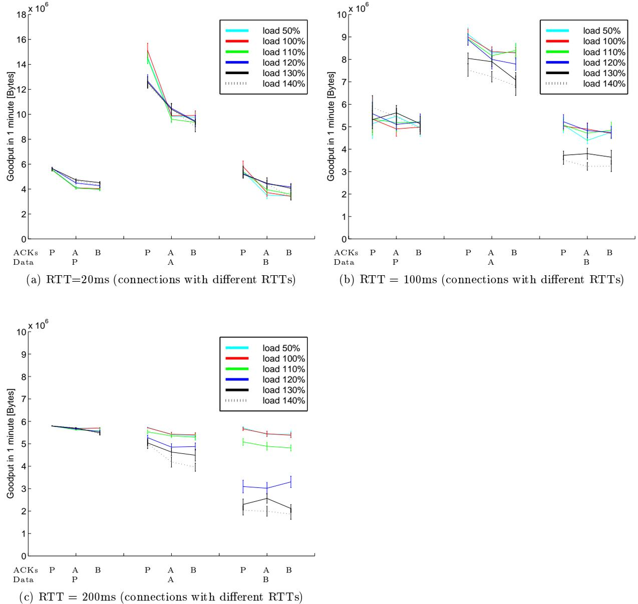
Figure 8: Comparison of goodput for different class combinations with varying load
