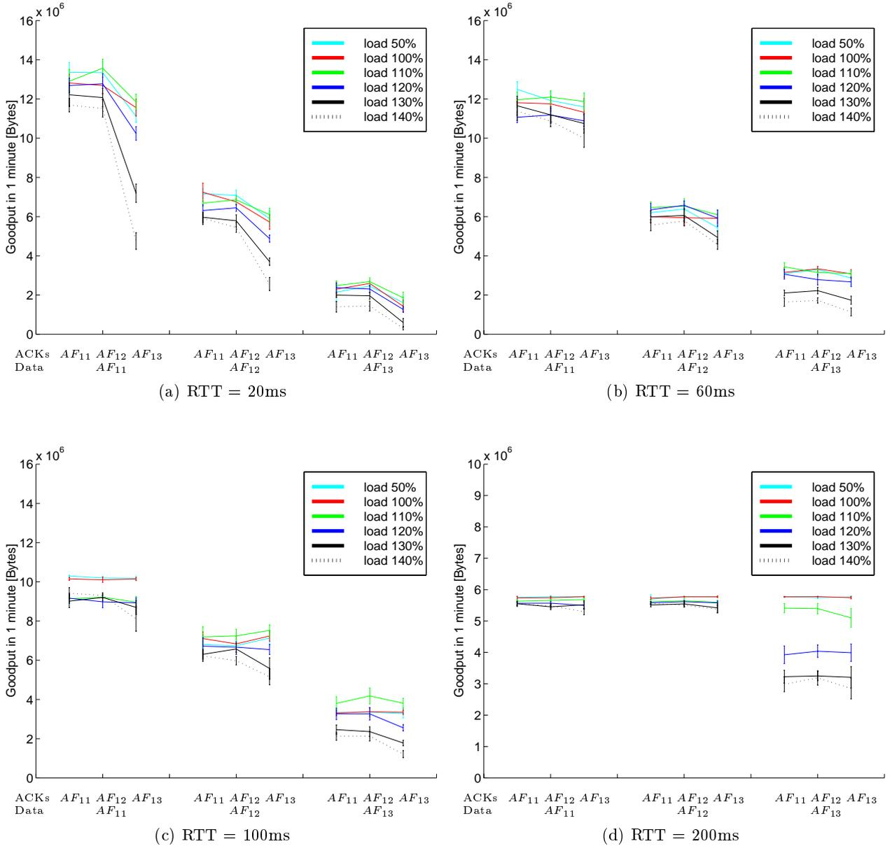
Figure 6: Comparison of goodput for different combinations of drop precedences with varying load
