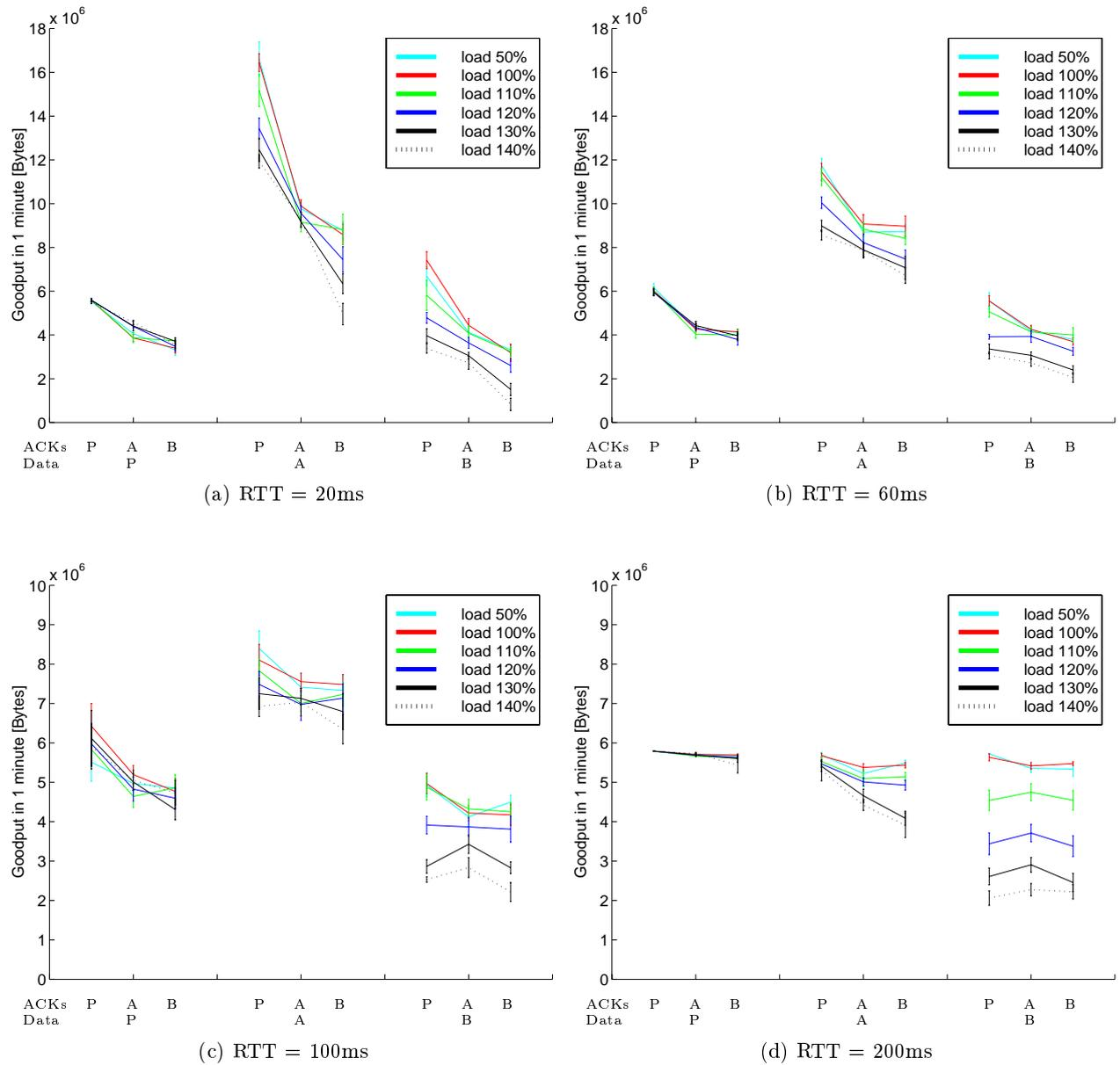
Figure 4: Comparison of goodput for different class combinations with varying load
