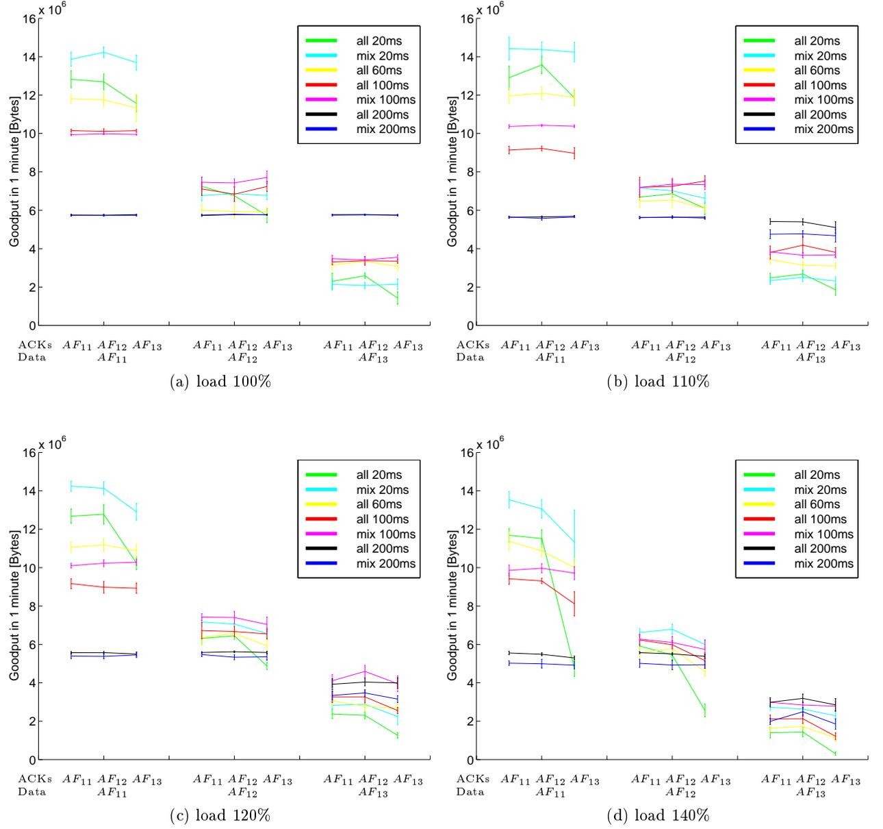
Figure 7: Comparison of goodput for different combinations of drop precedence with varying RTTs
