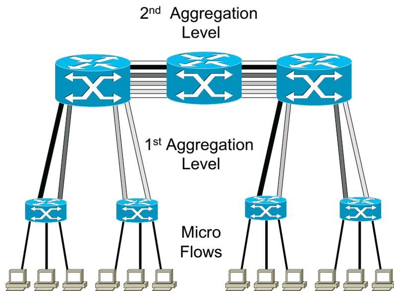
Figure 1: State reduction by hierarchical reservation aggregation.
