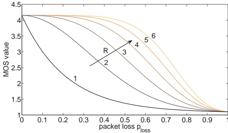
Figure 5: QoE in dependence on the replication degree (w/o jitter)
