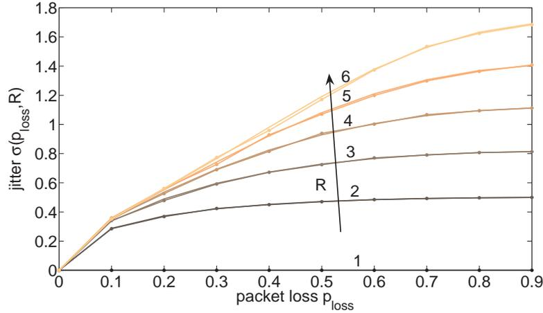
Figure 6: Increase of jitter due to replication of voice datagrams
