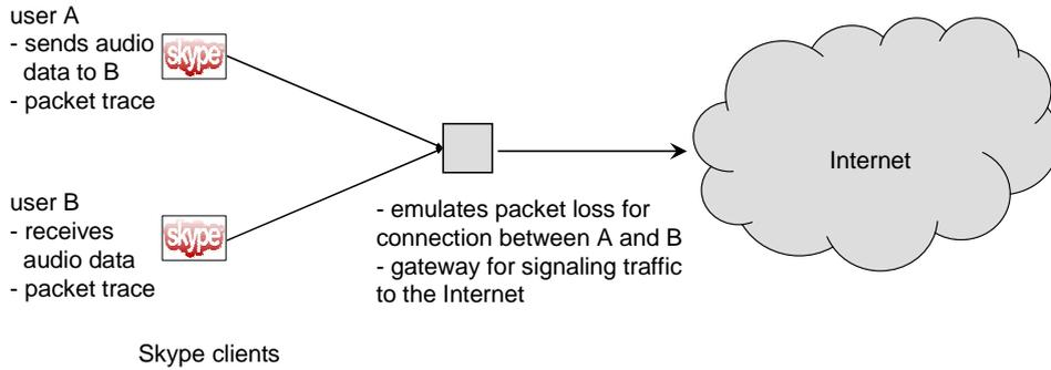
Figure 2: Measurement setup for a Skype call
