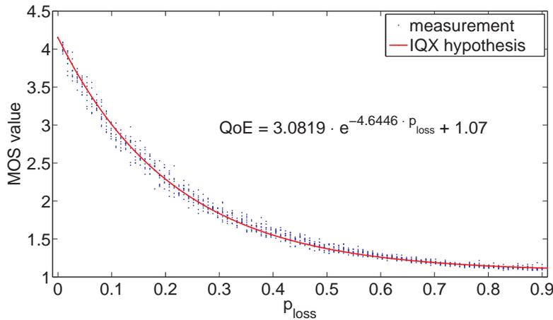
Figure 4: Exponential estimation of QoE in dependence of packet loss probability  $p_{loss}$
