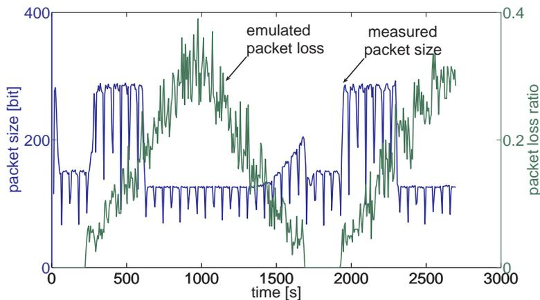
Figure 3: Measurement of Skype's QoE adaptation on changes in the end-to-end link
