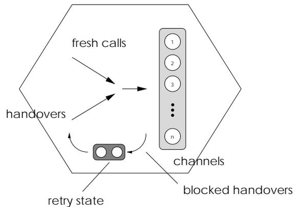
Figure 5: Handover retry mechanism
