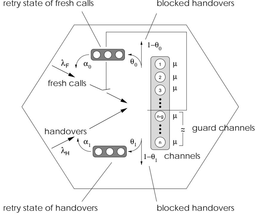
Figure 7: Analytical model of a cell with user redial behavior, guard channels and handover retry
