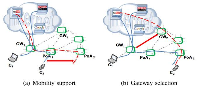
Fig. 1. Mobility support and resource management in wireless mesh networks
