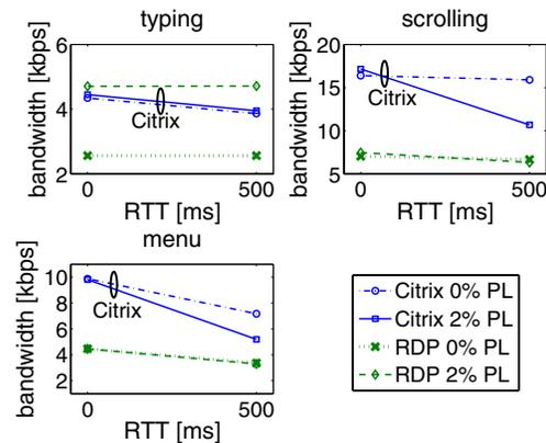
Fig. 6. Influence of network parameters on the bandwidth usage
