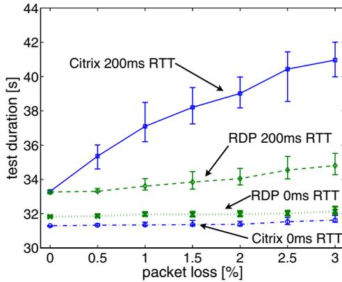
Fig. 9. Test duration using Word and varying packet loss
