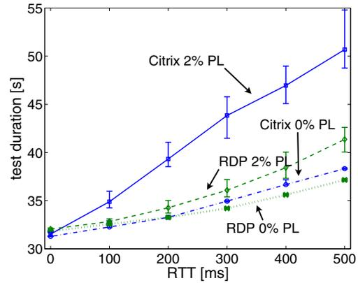
Fig. 7. Test durations using Word and different network delays
