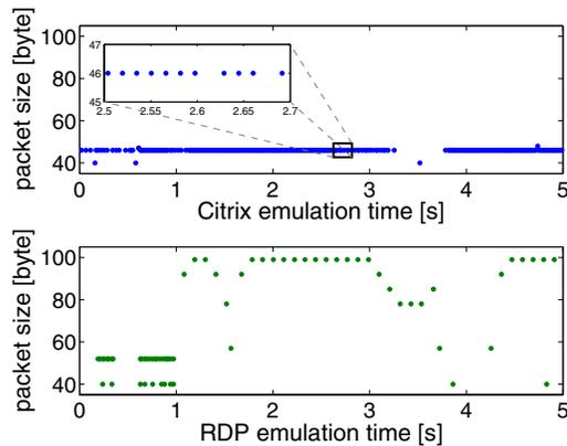
Fig. 3. Packet sizes sent by Citrix and RDP during the Word scrolling test.
