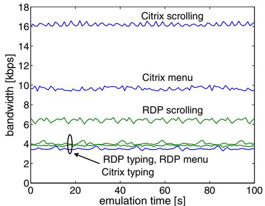
Fig. 2. Bandwidth used by the client for different MS Word tasks.
