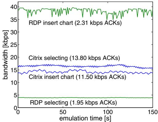
Fig. 4. Bandwidth used by the server for different Excel tasks.
