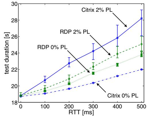
Fig. 8. Test durations using Excel and different network delays
