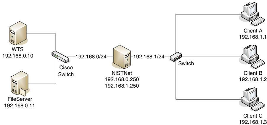
Fig. 1. Overview of the testbed environment
