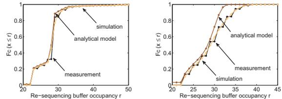
Fig. 5. Re-sequencing buffer occupancy for measurements, simulation and analysis
