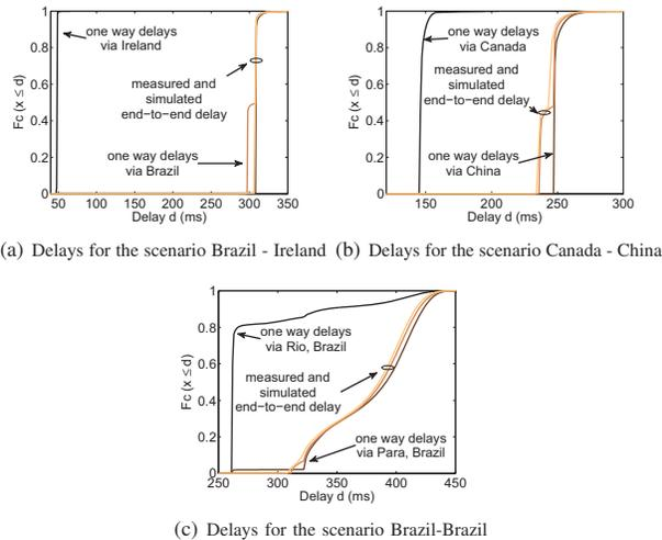
Fig. 9. Measured one way delays and end-to-end delays and simulated end-to-end delays for the investigated scenarios
