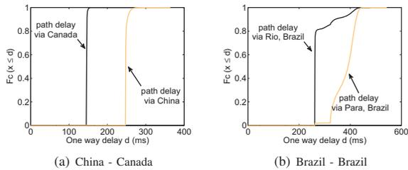
Fig. 4. Measured cumulative one way delay frequencies for the other scenarios
