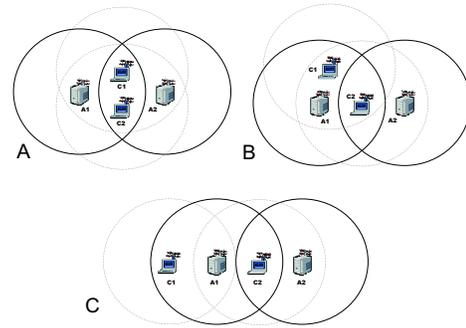
Fig. 1. Simulation Scenarios: overlapping cells
