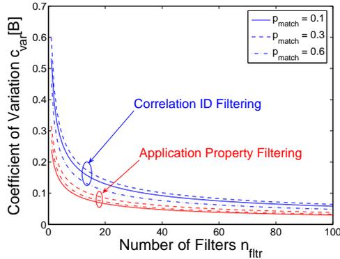
Fig. 9. Impact of the number of filters  $n_{filtr}$  and the match probability  $p_{match}$  on the coefficient of variation  $c_{var}[B]$  of the message processing time  $B$  for a replication grade  $R$  distributed according to a Binomial distribution.
