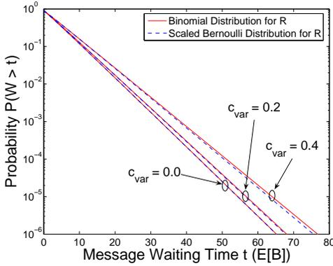
Fig. 11. Impact of the coefficient of variation  $c_{var}[B]$  and the distribution type of the message replication grade  $R$  on the complementary distribution function of the message waiting time  $W$  for a server utilization of  $\rho = 0.9$ .
