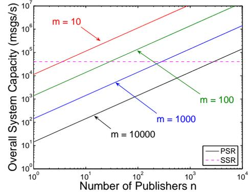
Fig. 15. Capacity comparison for publisher- and subscriber-side JMS server replication for a server utilization of  $\rho = 0.9$ , an average replication grade of  $E[R] = 1$ ,  $m$  subscribers, and correlation ID filtering.
