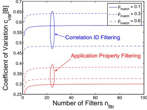
Fig. 8. Impact of the number of filters  $n_{filtr}$  and the match probability  $p_{match}$  on the coefficient of variation  $c_{var}[B]$  of the message processing time  $B$  for a replication grade  $R$  distributed according to a scaled Bernoulli distribution.
