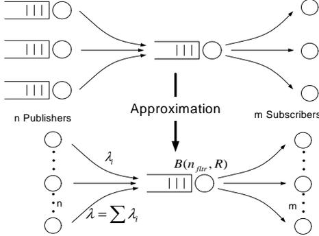
Fig. 7. A simple queueing model for a JMS server:  $M/G/1-\infty$ .
