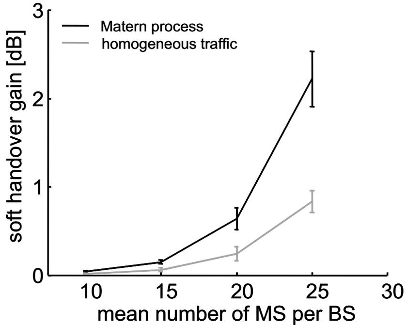
Figure 12: Comparison of the soft handover gain for homogeneous and inhomogeneous user distributions
