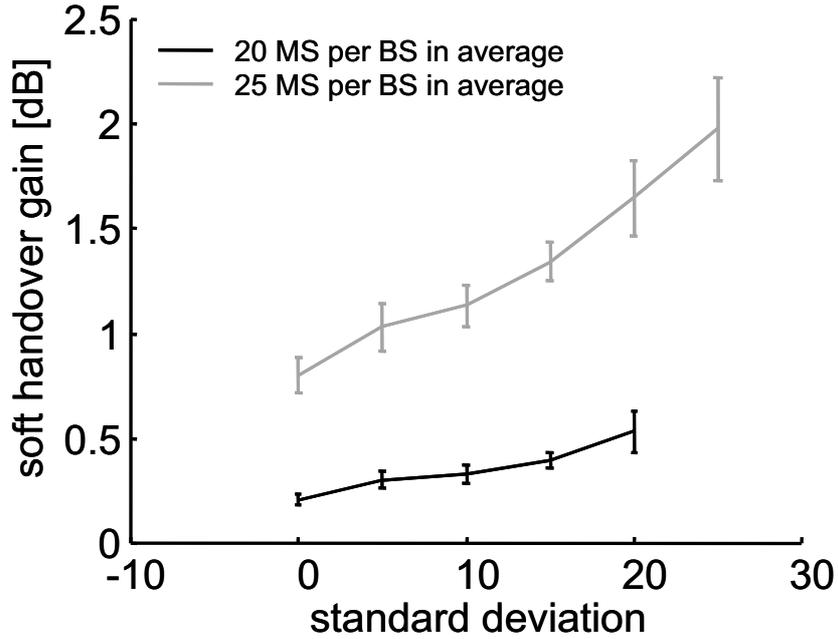
Figure 10: Soft handover gain for cell-wise inhomogeneous user density
