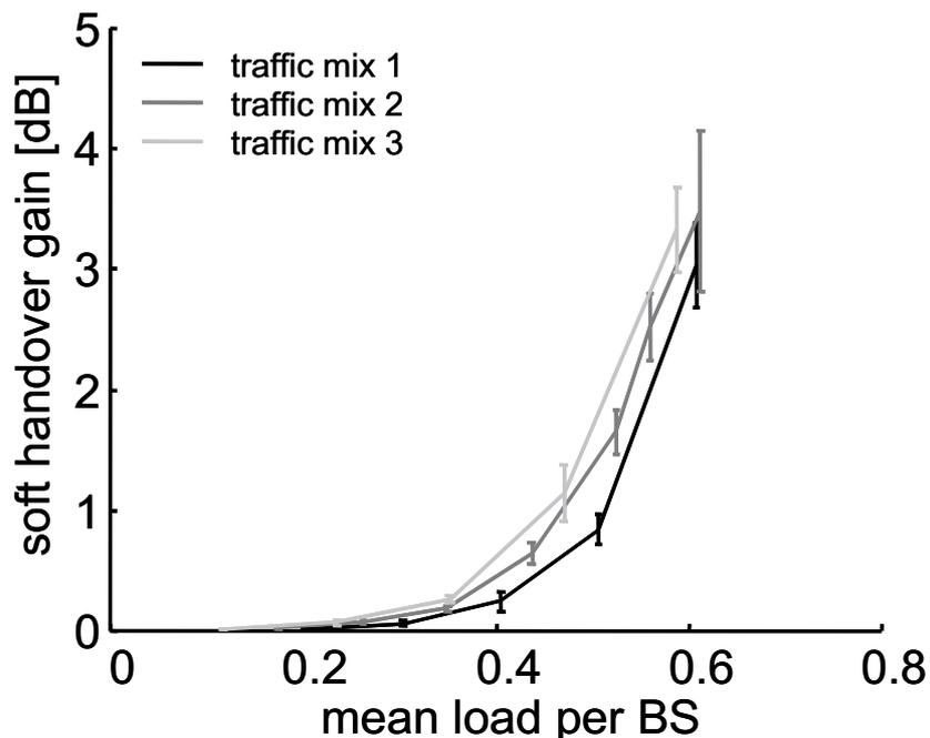
Figure 4: Soft handover gain versus BS load
