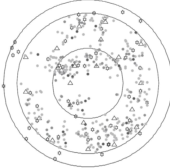
Figure 11: Inhomogeneous user distribution and irregular BS layout
