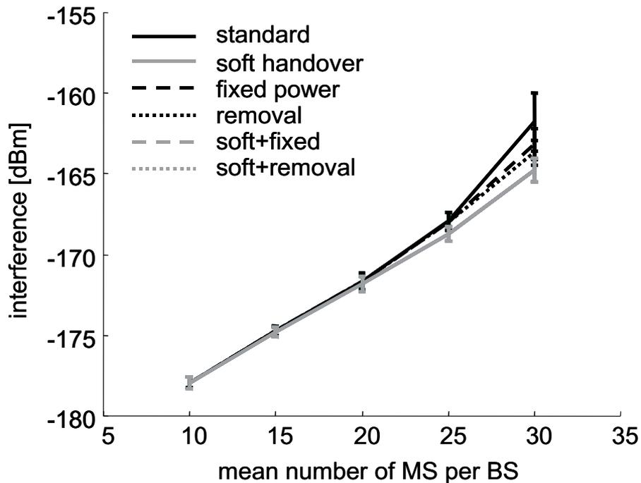
Figure 2: Mean interference depending on the user density
