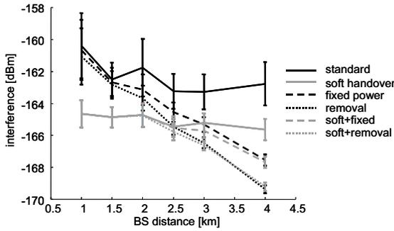
Fig. 4. Mean interference depending on the BS distance
