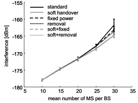
Fig. 2. Mean interference depending on the user density
