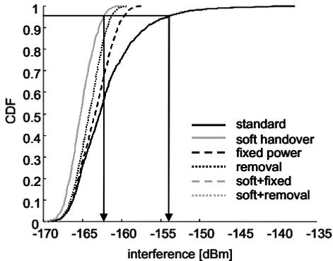
Fig. 5. CDF of the interference for different methods
