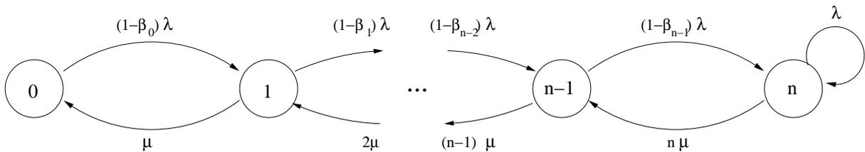
Figure 3: State diagram of a modified one-dimensional Markov chain
