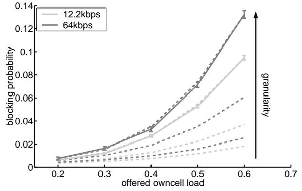
Figure 2: Approximation accuracy for different granularities
