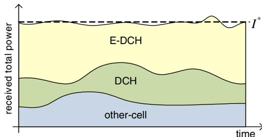
**Figure 1. RRM principle: E-DCH power adapts to DCH and other-cell interference**
