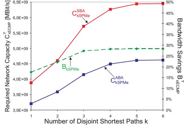
Figure 5: Network capacity requirements and bandwidth savings for  $kSPMe$  tunnels.
