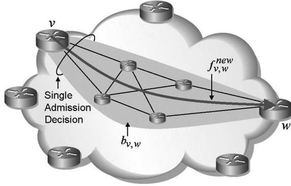
Figure 1: Network architecture with BBB NAC using multi-path capacity tunnels.
