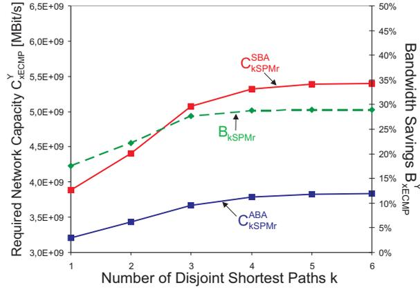
Figure 6: Network capacity requirements and bandwidth savings for  $kSPMr$  tunnels.
