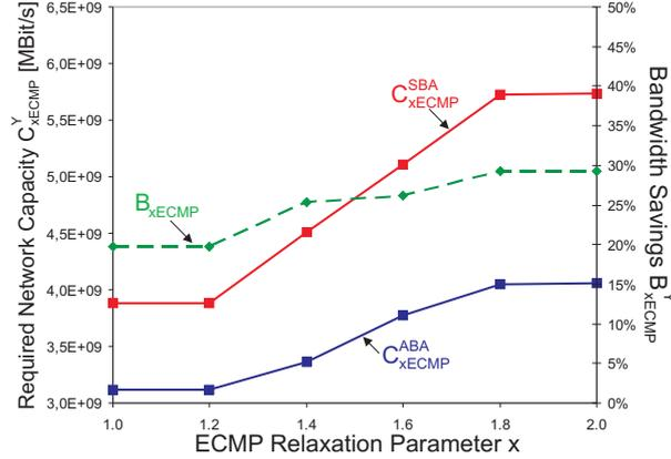
Figure 4: Network capacity requirements and bandwidth savings for  $xECMP$  tunnels.
