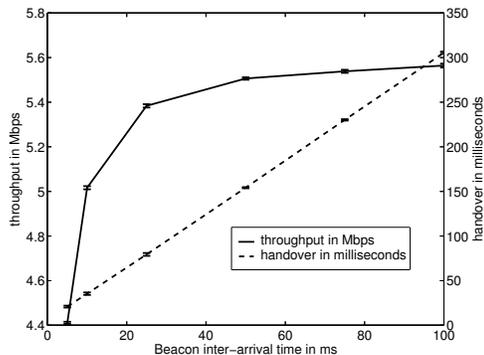
Fig. 6. Fast passive scanning with different Beacon inter-arrivals
