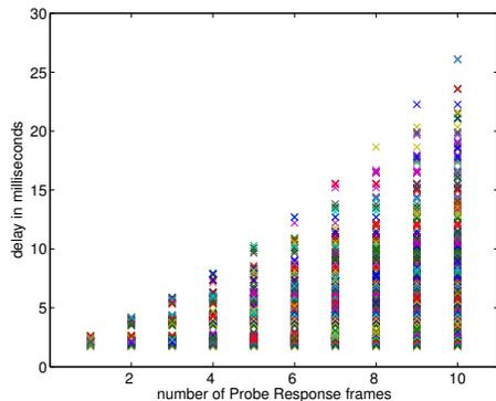
Fig. 7. Probe Response frame delay
