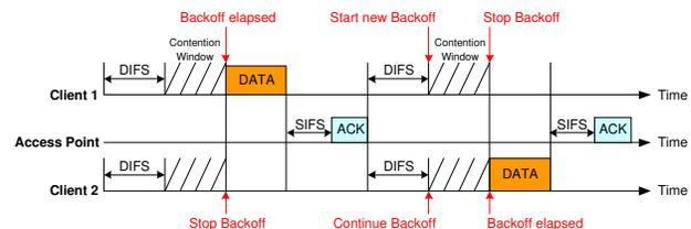
Fig. 1. Carrier Sense Multiple Access with Collision Avoidance
