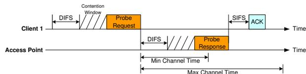
Fig. 2. Active scanning procedure
