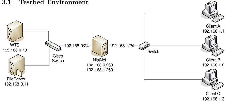
**Fig. 1.** Overview of the measurement setup
