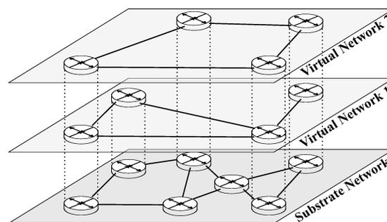
Fig. 1. Two virtual networks embedded in a substrate network.
