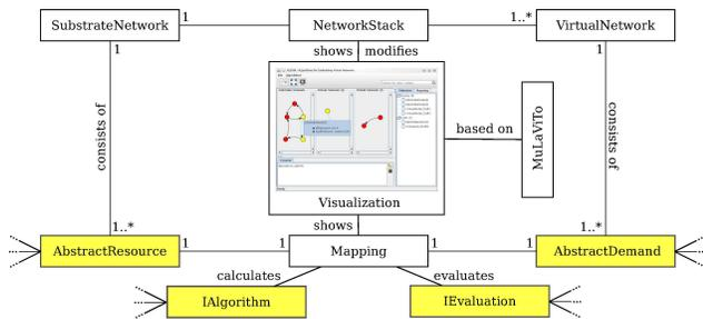
Fig. 2. The modular architecture of the ALEVIN software.
