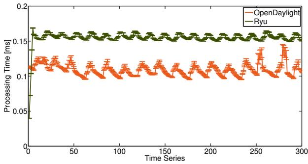
Fig. 2. Packet-out processing times for 20 unconnected switches.
