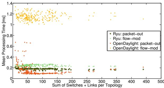
Fig. 6. Dependency of processing times on topology size.
