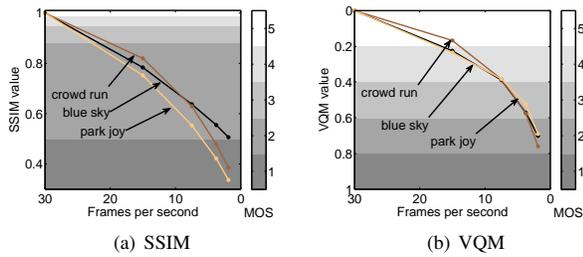
Fig. 5. Objective comparison of different frame rates
