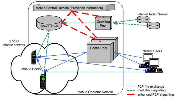
Figure 1. MNO-supported architecture
