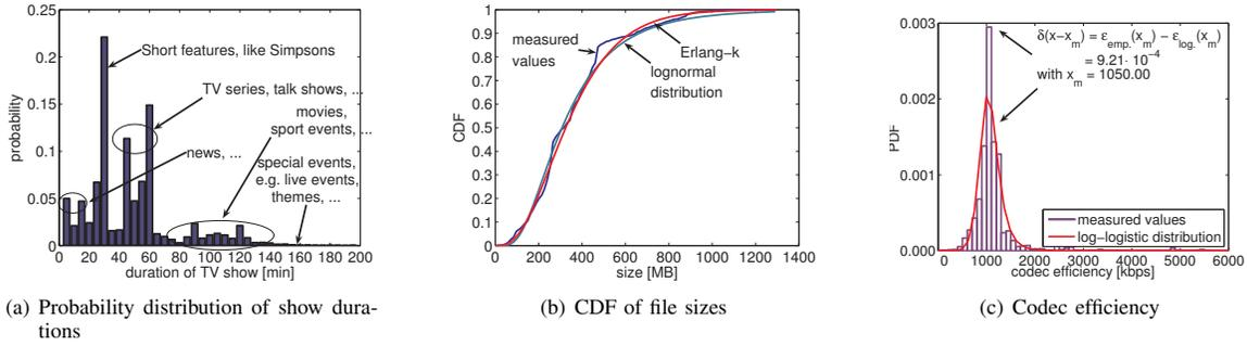
Fig. 1. Measured TV show durations, file sizes, and codec efficiency of OTR
