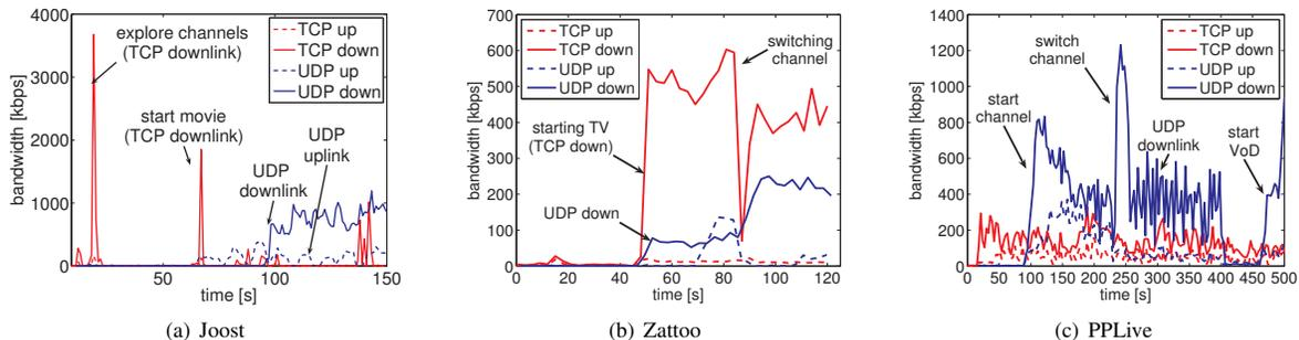
Fig. 3. Bandwidth consumption over time during P2PTV measurements
