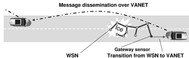
Figure 1: Hybrid Sensor-Vehicular Network
