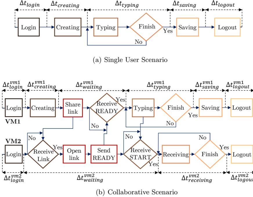
Fig. 2. Measurement Workflows
