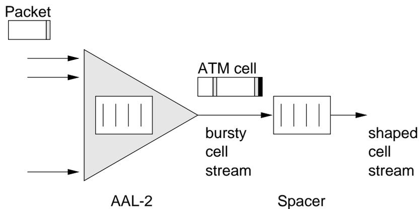
Figure 3: Model of AAL-2 combined with spacer
