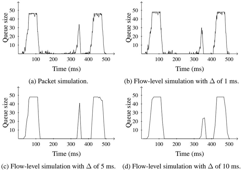
Figure 5: Queue sizes for packet-level simulation and flow-level simulation with different iteration intervals.
