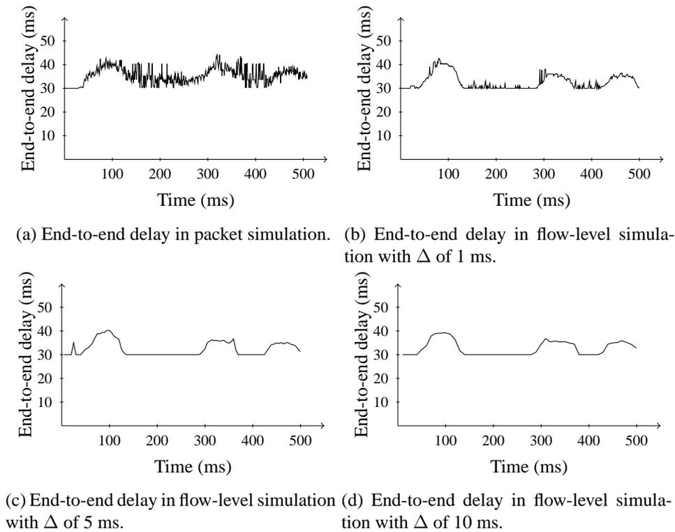
Figure 6: End-to-end delay statistics for the aggregate from 0 to 5.
