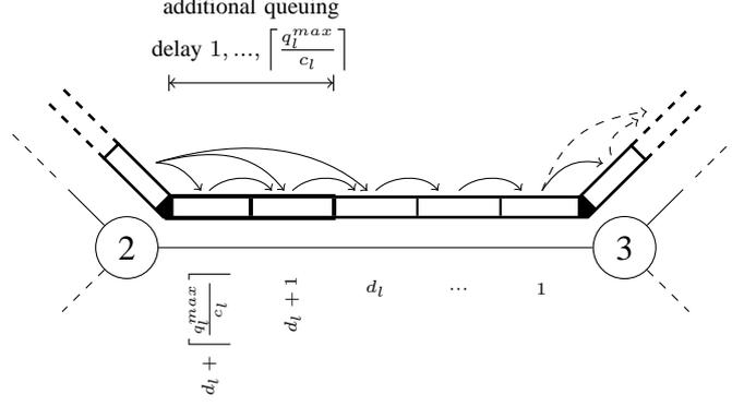
Figure 3: Array data structure for traffic aggregates with queuing delays.
