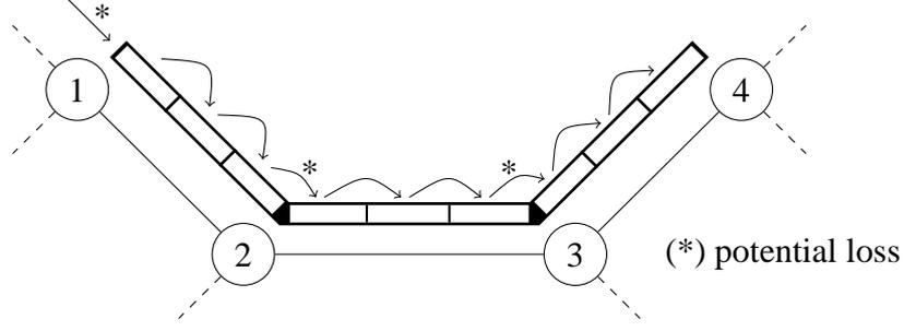
Figure 2: Network with 4 nodes and a traffic aggregate that crosses 3 links, each with a link delay of  $d_l = 3$ .
