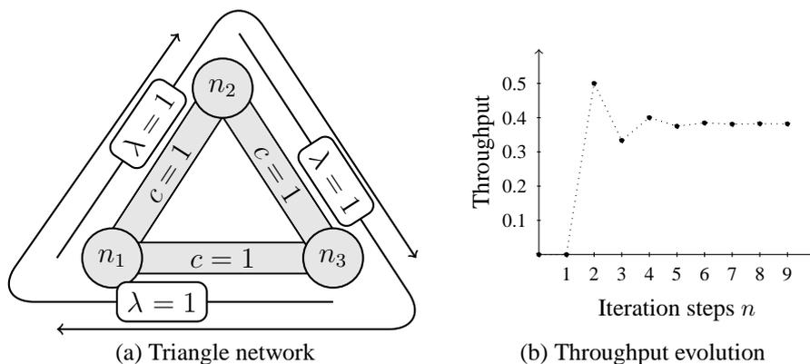
Figure 1: Throughput calculation for an triangle network.
