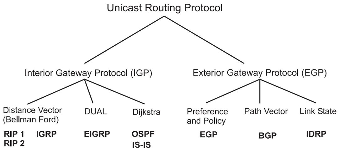
Figure 1: Overview of Unicast Routing Protocols
