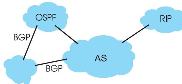
Figure 2: IGP (e.g. RIP, OSPF) protocols are used to route in an Autonomous System (AS). EGP (e.g. BGP) are used to route between AS.
