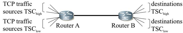
Figure 2: Single link simulation topology.
