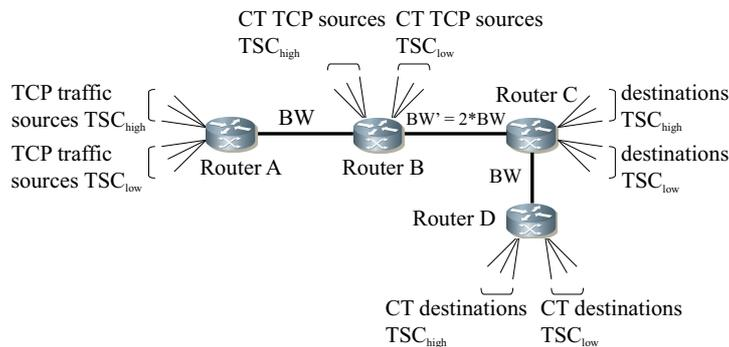
Figure 4: Multi link simulation topology.
