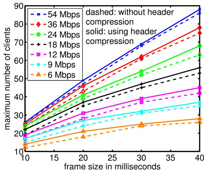
Figure 9: DCF using IEEE 802.11g data rates with and without header compression
