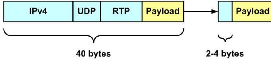
Figure 3: basic technology of header compression
