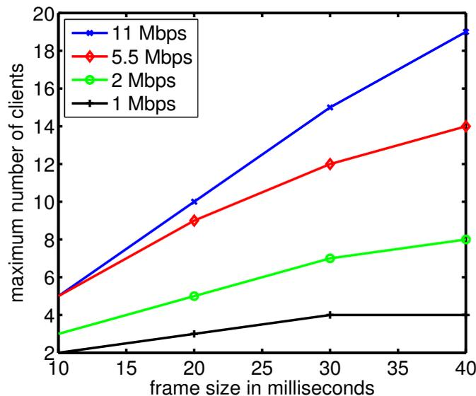
Figure 5: DCF using IEEE 802.11b data rates
