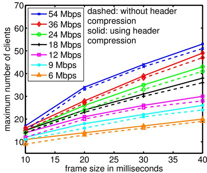
Figure 10: EDCA using IEEE 802.11g data rates with and without header compression
