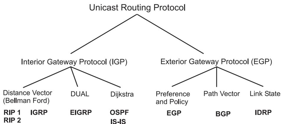
Figure 1: Overview of Unicast Routing Protocols
