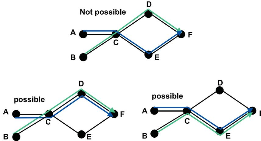
Figure 2: IP Routing restriction
