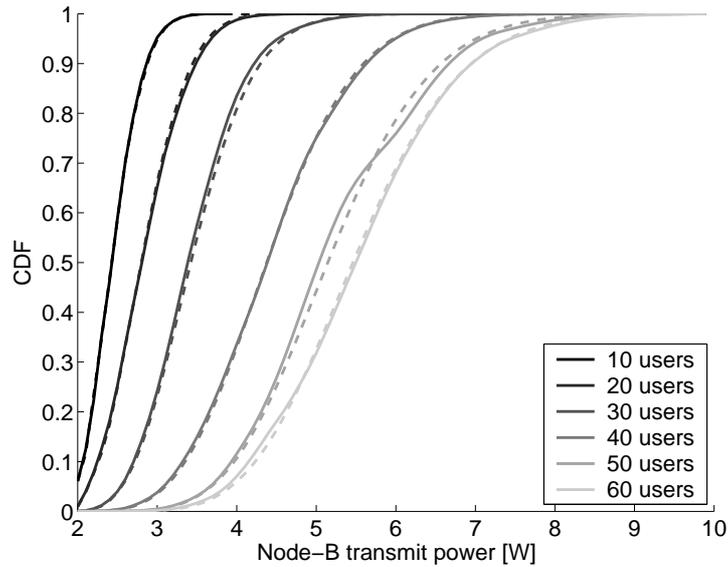
Figure 4: Comparison of the approximative power control algorithm and the exact implementation of the UMTS power control mechanism
