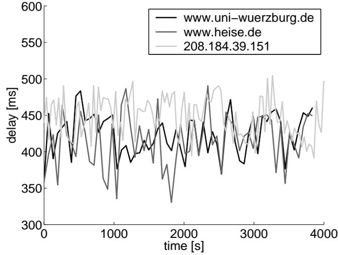
Figure 3: Delay for the transmit time between the NodeB and a WWW server in the Internet.
