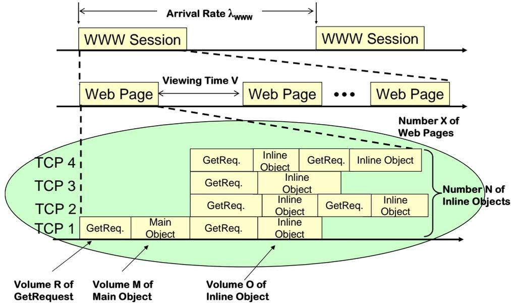
Figure 1: Web traffic model is structured into session, page, and TCP layer
