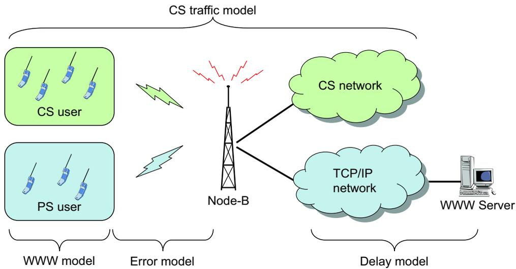
Figure 2: UMTS scenario is described by a given CS traffic and a composed WWW traffic model.
