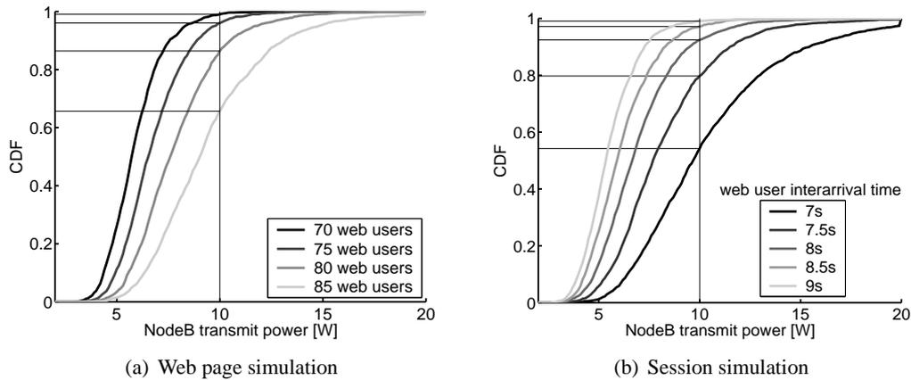
Figure 10: Outage occurs if the NodeB transmit power exceeds 10 W
