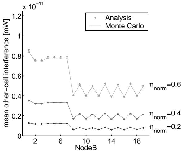
Fig. 2. Mean other-cell interferences in a hexagonal cell layout
