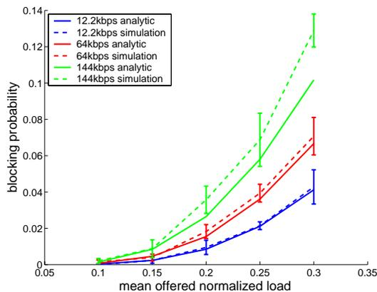
Fig. 4. Blocking probabilities for three service classes
