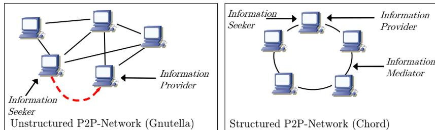
**Fig. 3.** Unstructured and structured P2P overlay topologies
