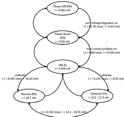
Figure 1: Simplified state machine of CC2420
