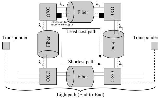
Fig. 1. MODEL OF OPTICAL TRANSMISSION AND OPTICAL COMPONENTS
