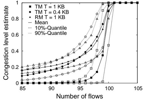
Figure 6: Marking with early warning (MEW): CLEs should gently increase up to 1 if the traffic rate is below the virtual queue rate and stay at 1 if it is above.
