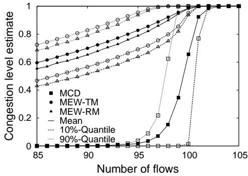
(e) Increased burstiness:  $E[A] = 100$  ms and  $E[B] = 300$  bytes instead of  $E[A] = 20$  ms and  $E[B] = 60$  bytes.
