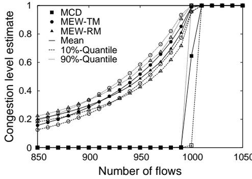
(c) Increased aggregation level: capacity for  $n = 1000$  flows instead of  $n = 100$  flows.
