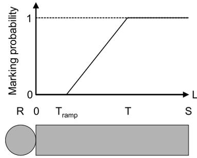
Figure 2: The ramp marker marks all packets if the length of its virtual queue exceeds its threshold  $T$ , but it also marks packets probabilistically between  $T_{ramp}$  and  $T$ .
