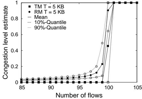
Figure 5: Marking with clear decisions (MCD): CLEs should be 0 if traffic rate is below the virtual queue rate and 1 if it is above.
