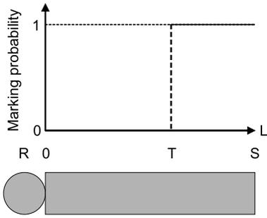
Figure 1: The threshold marker marks packets if the length of its virtual queue exceeds its threshold  $T$ .
