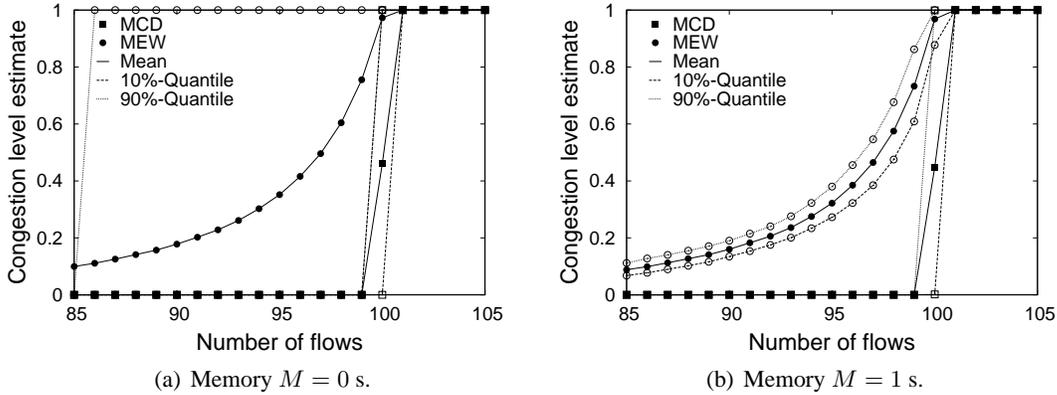
Figure 7: The congestion level estimator’s memory influences the stability of the CLE (threshold marking with  $S = 15$  KB and  $T = 5$  KB or  $T = 1$  KB, respectively).
