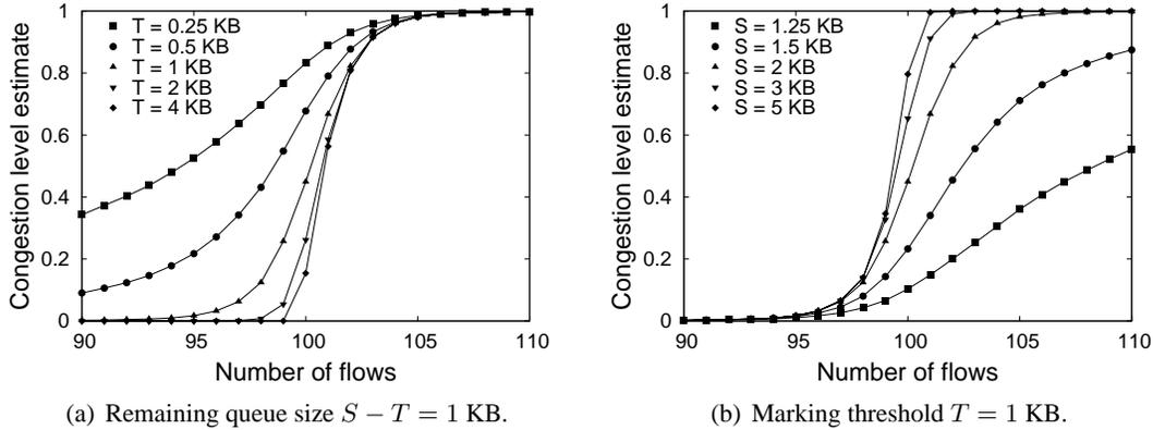
Figure 4: CLE for threshold marking with variable queue sizes  $S$ .
