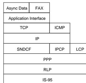
Fig. 1. Wireless CDMA protocol stack
