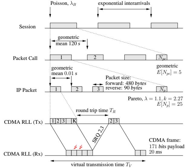
Fig. 2. CDMA user connection process
