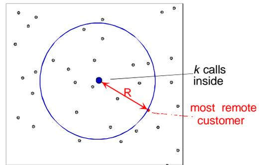
*Fig. 5: CDMA cell with  $k$  supported users*
