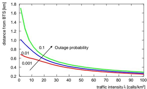
**Fig. 15: CDMA traffic based network planning**
