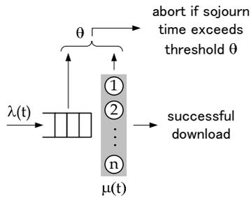
**Fig. 3.** Model of server-based content distribution system
