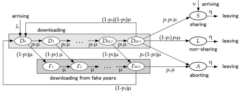
**Fig. 1.** Flow diagram of P2P file sharing model
