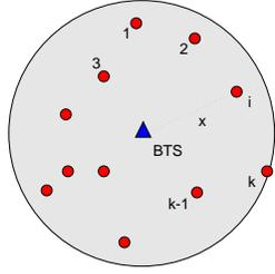
Figure 1: CDMA cell with  $k$  supported calls
