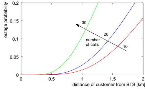
Figure 5: Impact of customer-BTS distance on outage probability
