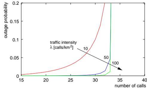
Figure 7: Relationship between capacity and outage probability
