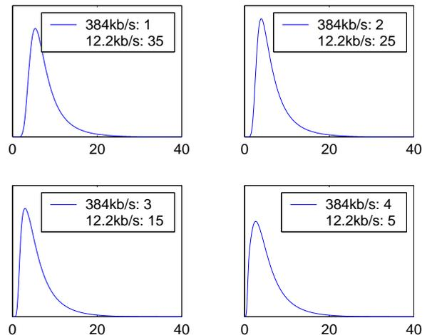
Fig. 2. Pmf of the noise rise [dB] in a two-services environment. The legend contains the means of the numbers of active subscribers for the various services.
