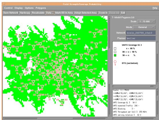
Fig. 3. A realistic network in Cologne. Colored is the area with more than 90% coverage probability for a 144kb/s UMTS service.
