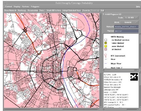
Fig. 4. The same network. The colored area shows where parts of the expected traffic of the 144kb/s UMTS service are blocked.
