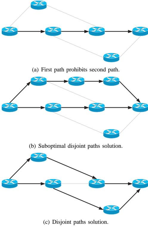
Fig. 2. The iterative application of the shortest path algorithms cannot find shortest disjoint paths in some cases.
