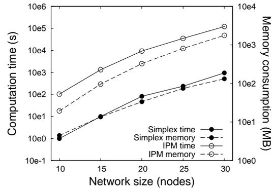
Fig. 4. Comparison of memory consumption and computation time for the Simplex and an interior point method for networks of different size.
