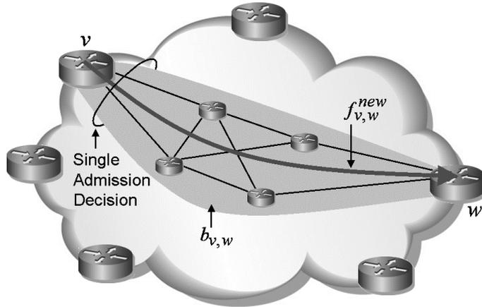
Figure 1: Network architecture with BBB NAC
