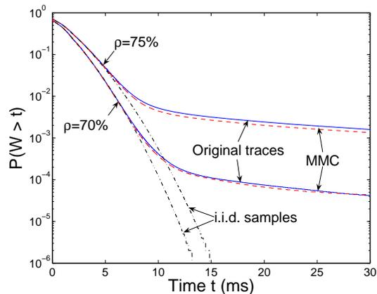
**Figure 5:** Validation of different traffic models for the iSAC codec with original traces using the waiting time of multiplexed sources.
