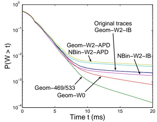
**Figure 3:** Validation of different traffic models for the G.723.1 codec with original traces using the waiting time of multiplexed sources.
