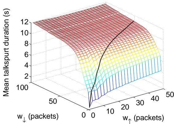
**Figure 2:** Impact of the window parameters  $w_{\downarrow}$  and  $w_{\uparrow}$  on the measured mean duration  $E[D_{on}^{real}]$  of the on-phases for the G.723.1 codec.
