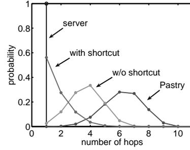
Fig. 3. Hop count distribution for a central server system, an unmodified Pastry, and our modified Pastry both with and without shortcut link.
