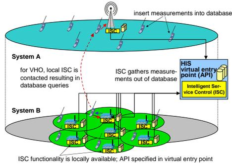
Fig. 1. Distributed information system: the database consisting of measurements is distributed among APs together with the ISC (enhanced from [7])
