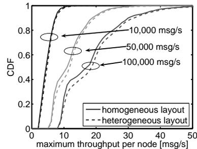
Fig. 6. CDF of maximum message throughput for homogeneous and heterogeneous network layouts.
