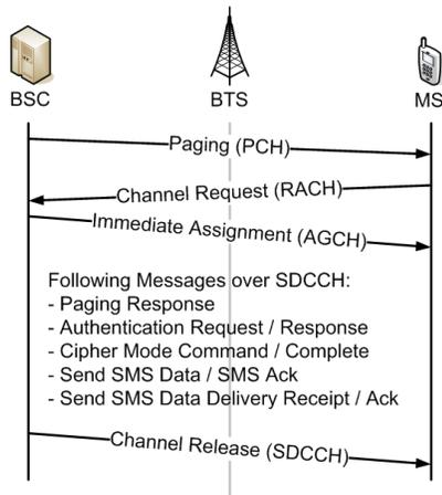
Fig. 2. Air interface channels used for SMS-MT
