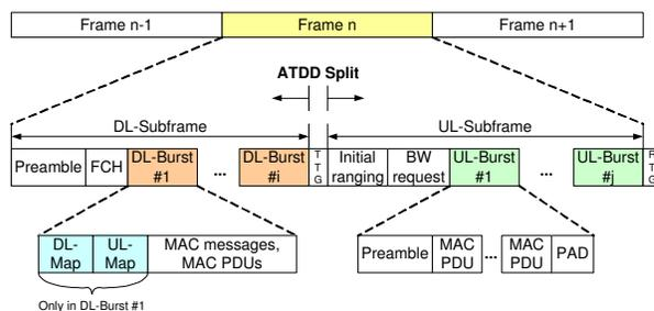
Fig. 1. WiMAX TDD frame structure
