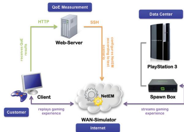
Fig. 1. Testbed Setup - Logical View
