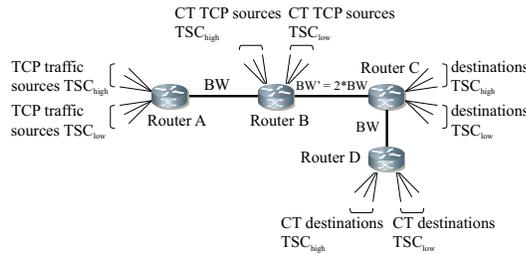
**Figure 4.** Multi link simulation topology
