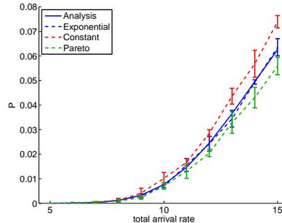
**Figure 8.** Sensitivity of the dropping probabilities against volume size distribution.
