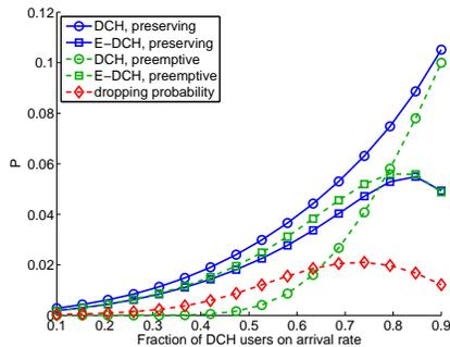
**Figure 7.** Impact of preemption depends on ratio between DCH and E-DCH users.
