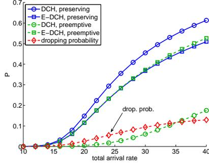
**Figure 5.** Blocking and dropping probabilities for QoS and E-DCH users
