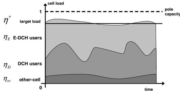
**Figure 1.** Illustration of the RRM principles for the E-DCH best-effort service.
