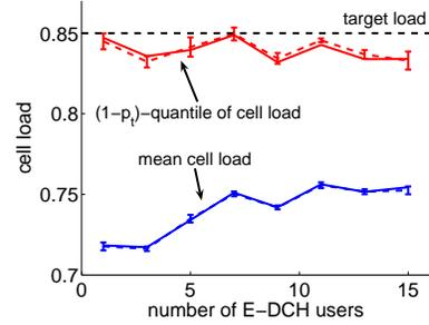
**Figure 4.** Mean cell load and 95%-quantiles.
