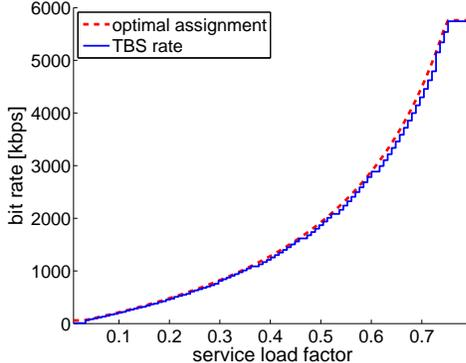
**Figure 2.** Mapping of service load factors to bit rates
